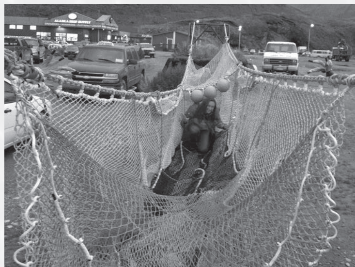
YRDLA Policy Director Becca Robbins Gisclair tries following the path of a salmon escaping from a salmon excluder. The excluders allow salmon to escape from pollock nets while keeping the pollock in, and many pollock boats use these as part of their gear. Dutch Harbor, AK.
